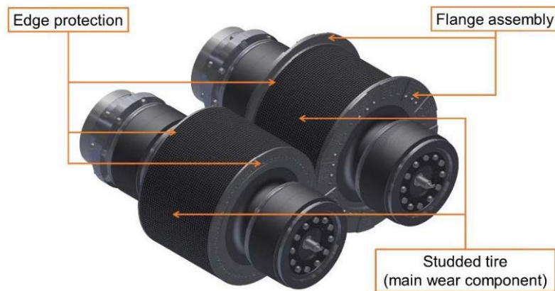
Figure 24 – A diagram showing the flange assembly of the Metso HRC® HPRG (diagram sourced from: Herman et al. 2015, "Building the world's largest HPGR – the HRC™ 3000 at the Morenci Metcalf Concentrator" SAG Conference, Vancouver).
