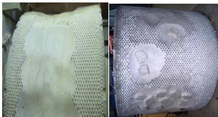
Figure 26 – Photographs showing HPGR roll “washout” as a result of poor inspection and stud maintenance (source: Koski, S., et al., 2011. Cerro Verde concentrator - four years operating HPGRs, SAG 2011. Department of Mining Engineering, University of British Columbia, Vancouver, B. C., Canada; and Burchardt, E, Patzelt, N., Knecht, J. and Klymowski, R.,;(2011), HPGR's in Minerals : What do existing operations tell us for the future?, Paper #108, SAG 2011. Department of Mining Engineering, University of British Columbia, Vancouver, B. C., Canada. Burchardt, E (2013) HPGRs in Hard Rock Mining, Mining Magazine).
