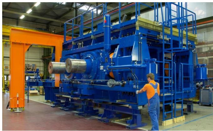
Figure 21 – A photograph showing a Weir/KHD HPGR design
