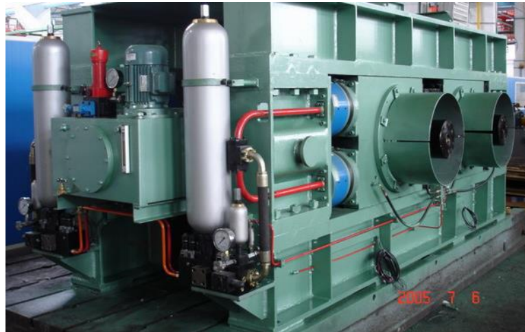
Figure 22 – A photograph showing the Citic-HIC HPGR roll designs with Nitrogen hydraulic spring system
