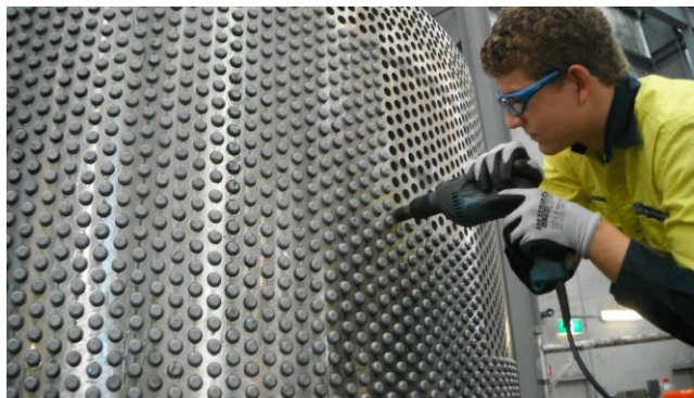
Figure 17 – A photograph showing stud re-lining and maintenance being performed by hand.
