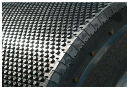
Figure 12 – A photograph of a Weir/KHD HPGR with a studded surface and edge protection.
