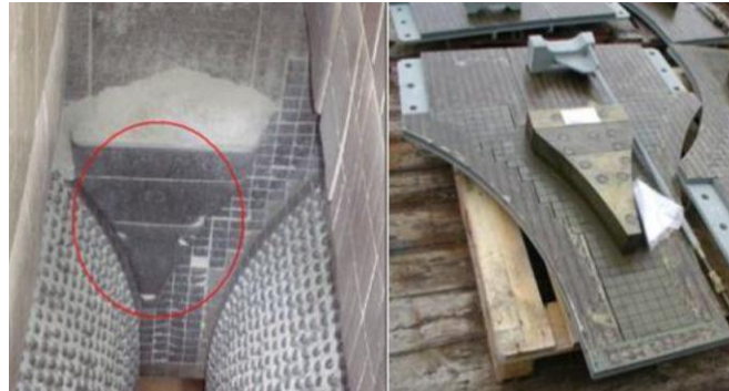
Figure 13 – Photographs showing cheek plates that protect the roll edges from side wear.
