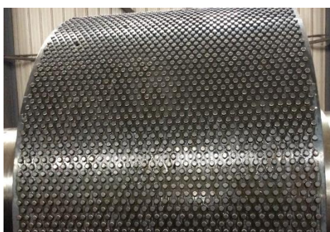
Figure 8 – A photograph of an early model HPGR from Weir/KHD without edge protection.
