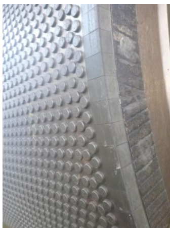
Figure 19 –A photograph of the Polysius surface and edge design.
