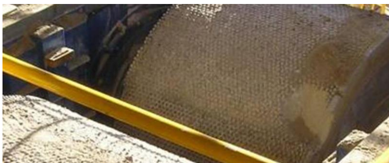
Figure 18 – A photograph showing Polysius HPGR with “washout” in the form of severe edge wear.
