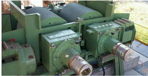
Figure 9 – A photograph of the Weir/KHD HPGR roll designs without edge protection from the Argyle diamond mine.
