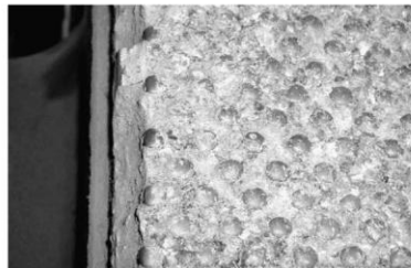
Figure 10 – A photograph showing edge wear on new Weir/KHD roll designs.
